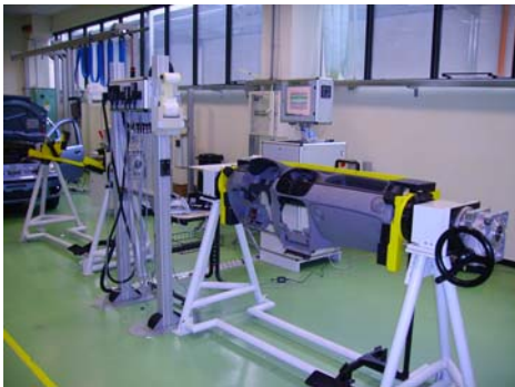
Fig. 6: Test stand for Instrument board
