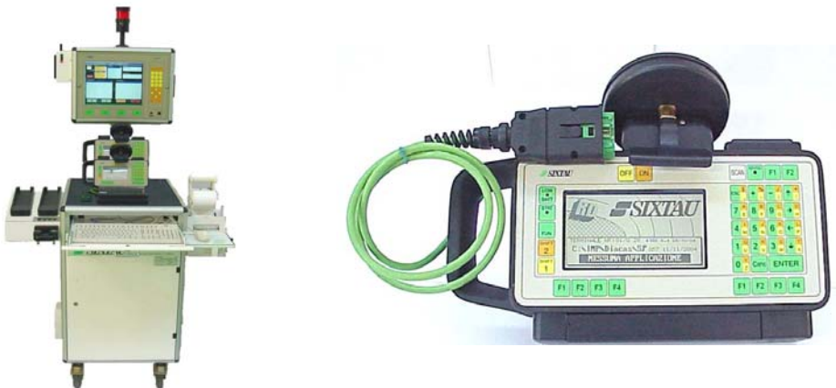
Fig. 9: Stand for final testing on the end of the process final assembly
