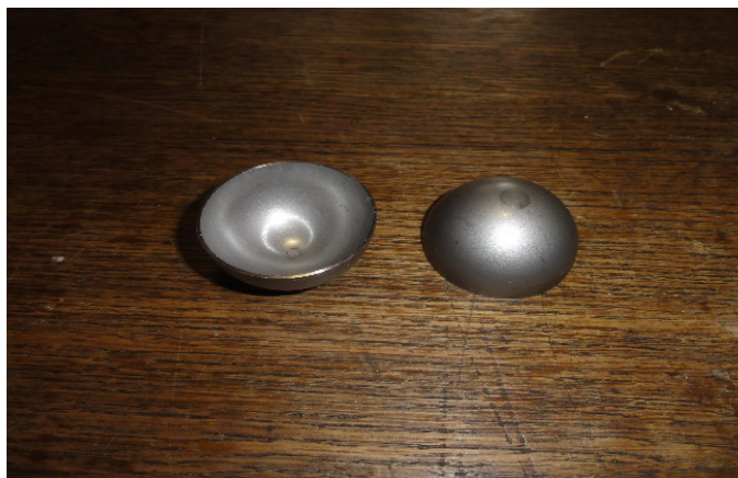
Figure 1: Inox sphere \phi 60 after pressing (Source: Miljan Miletic)
